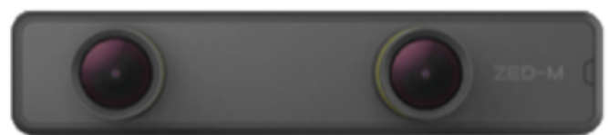
Figure 12. Zed Mini Stereo Camera [9] which was placed on the VR Oculus Rift device during NASA JSC test week.
