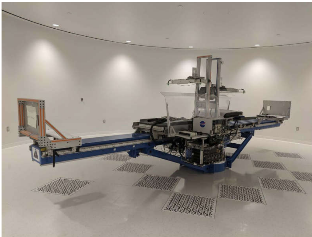
FIGURE 1: Short Radius Centrifuge, located on the Texas A&M University Campus at the Human Clinical Research Facility. Subjects will perform a bimanual movement or force coordination task at 0, 0.25, 0.5, 0.75, 1, and 1.8 G.
